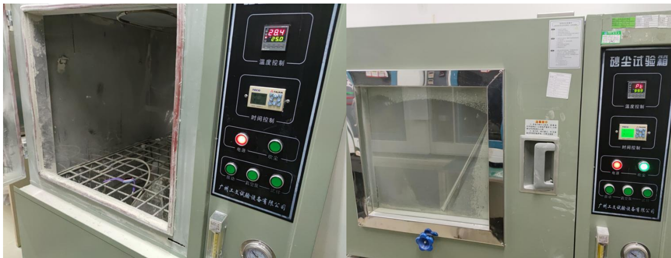
Photo 3: IP6X test of model KW1401
