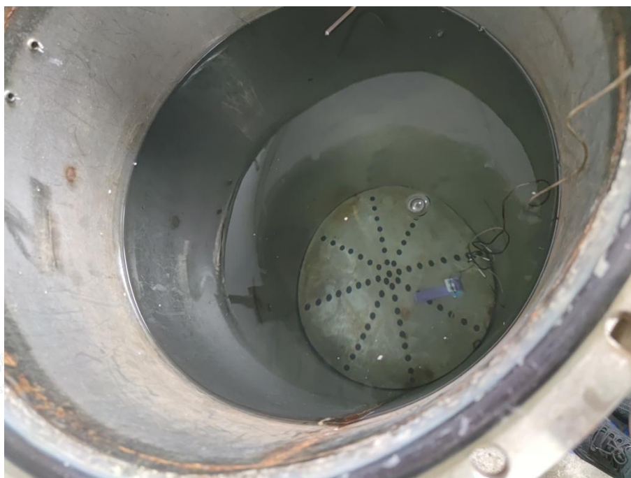
Photo 4: IPX8 test of model KW1401
